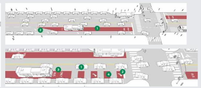
Transit Approach Lane (top) and Queue Bypass (bottom); green numbers highlight pavement marking features. Source: NACTO
