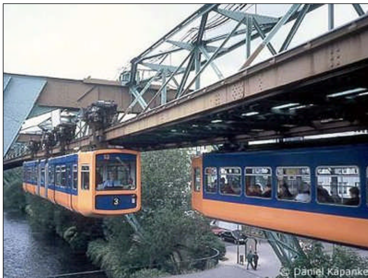
Figure 3.9 – Suspended Monorail in Wuppertal, Germany
