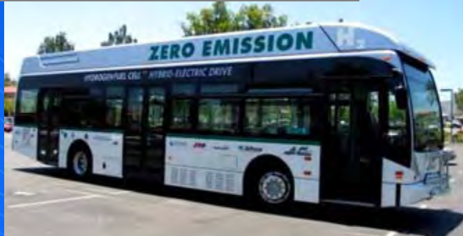
Van Hool A330 with ISE ThunderVolt TB-40FCH fuel cell hybrid-electric drive
