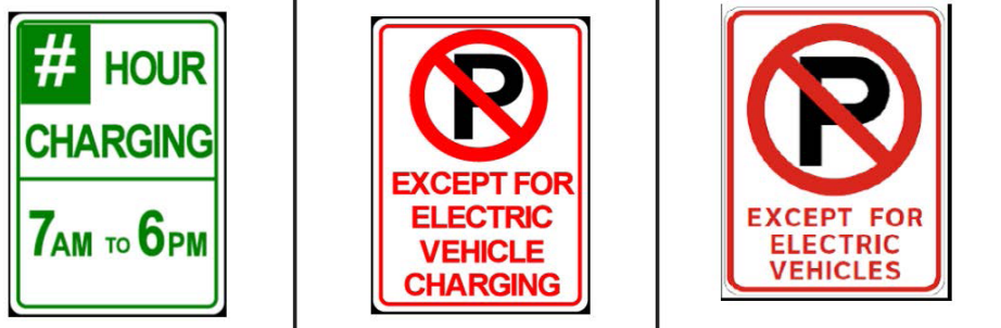
Figure 13.3: Candidate regulatory signs for PEV charging
